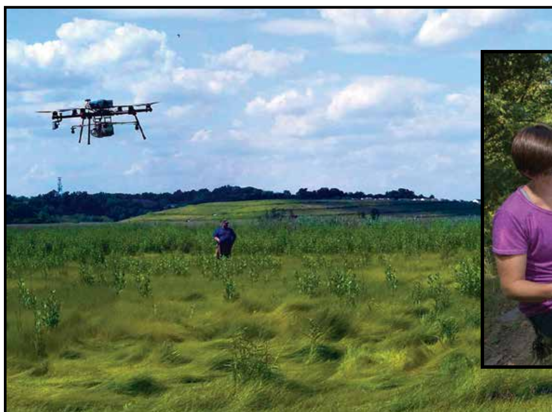
Drone, applying liquid larvicide to control mosquitoes.
